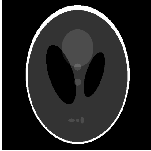
Figure 1: The analytical phantom sampled on a 1024 \times 1024 grid.
